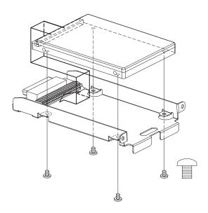
4. Slide the Tray with Hard Disk Drive into the slot and press it firmly to ensure secure connection. Tighten the two screws back that have been removed in Step 2. Place the Front Cover back and tighten the four screws back that have been removed in Step 1.
