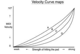
05. Select the Velocity curve field and adjust the Velocity curve while hitting the Pad.
