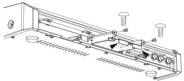
3. Connect 50 pin connector of Hard Disk Drive to 50 pin connector of the Tray as illustrated, and press it firmly to ensure secure connection.
