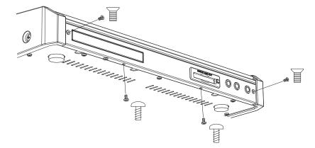
2. Remove the two screws for Internal Hard Disk Drive Tray and remove the Tray with your fingers at the **b** marks.
