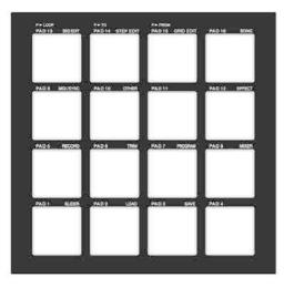
The MPC2500 has 16 drum pads. The pads perform various function besides making sounds when hit. In this section, you will learn about various functions of the pad.
