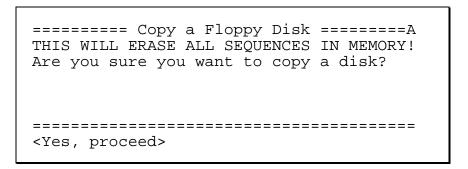
The disk copy function requires the use of the sequence memory and therefore will erase all existing sequences before making the copy. Be sure to back up your sequences to disk before executing the Copy Disk utility. If it's OK to erase all sequence data, press <Yes, proceed> to proceed with the copy function. A series of messages will be subsequently presented, instructing you to alternately insert the source and destination disks in order to make the copy.
